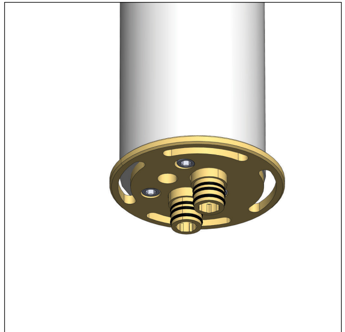
Ensure double o-rings are undamaged and greased
