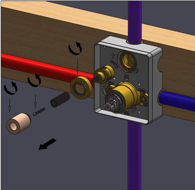
1. Remove diverter cover by turning with hand
