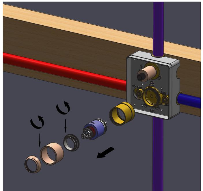
**INSTALLING EXTENSIONS TO THE VALVE - OPTIONAL**
