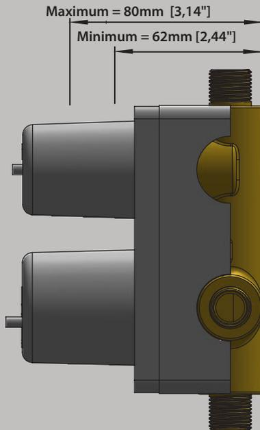
The distance between back of the valve to the finished tile surface should be between 2.44 and 3.14 inches.
