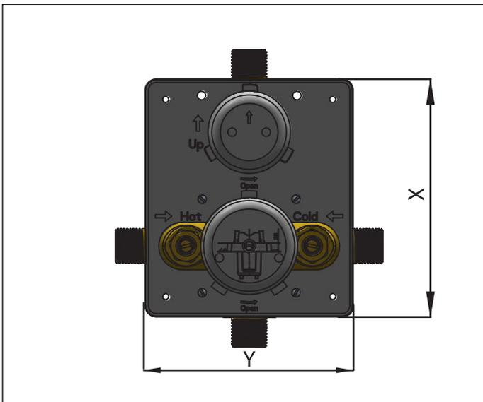
Isenberg's PBV1005A valve comes with a pre-attached mud-guard. This mud-guard is not to be removed or discarded. Its purpose is to guide the installation professional on the proper cut-out dimensions of the drywall.
