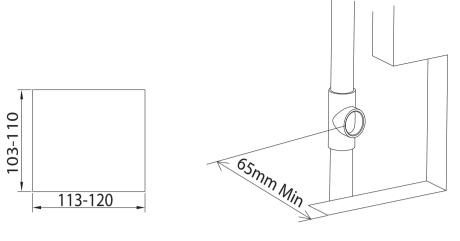
3. Create a cut out in the wall of the appropriate size
