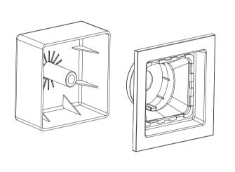
9. Lock the main body on the connector with the M4x20 Screws
