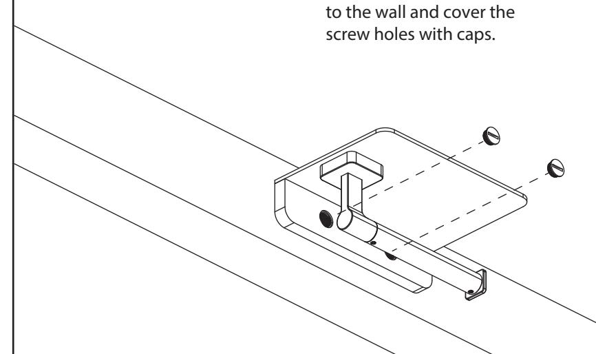
4. Fix the toilet paper holder to the wall and cover the screw holes with caps.
