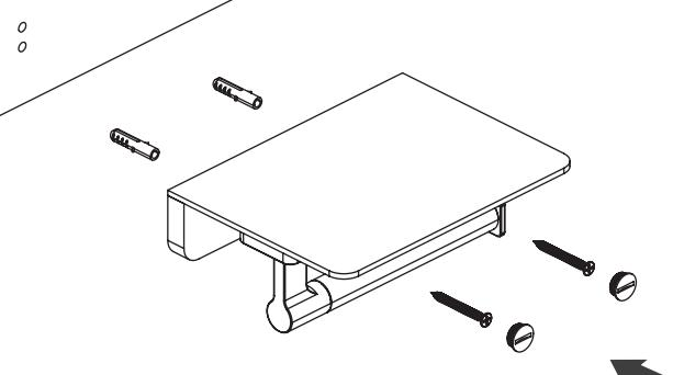
3. Insert wall plug and fix the screw in to the wall
