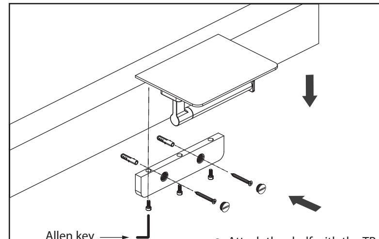
2. Attach the shelf with the TP holder to the flange using screws, and tighten them with an Allen key.
