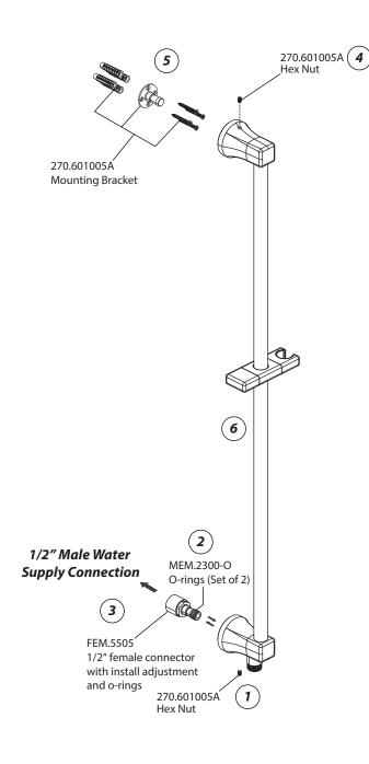
1. Loosen & remove two hex screws using 1.5mm Allen key.
