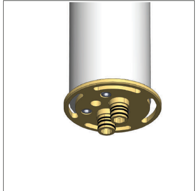
Ensure double o-rings are undamaged and greased
