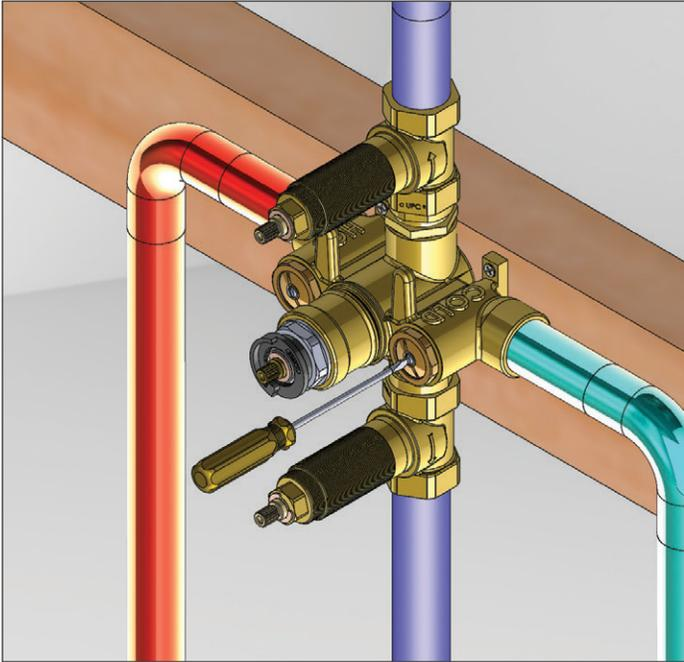
In order to remove the supply stops do not twist the screw in the middle of the supply stop
