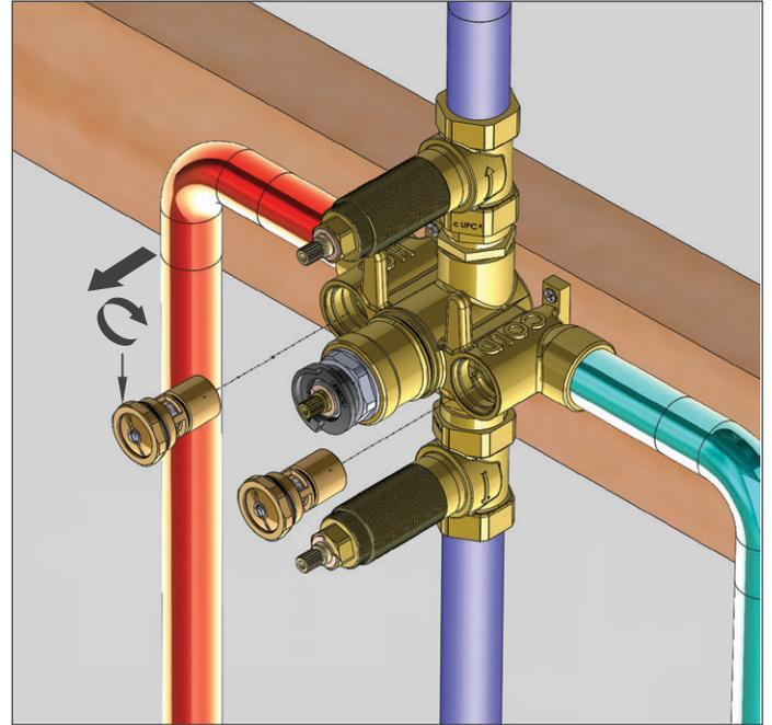
Use a spanner to twist in the shown position and remove supply stop
