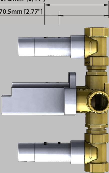
The distance between back of the valve to the finished tile surface should be between 2.77" and 3.44" inches.
