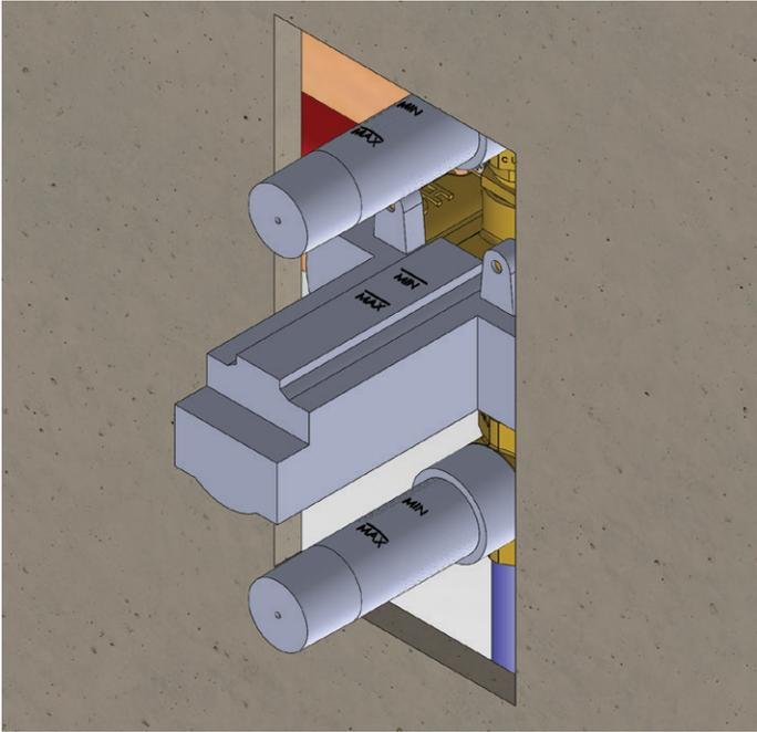
Install Drywall and Tile. Ensure finished tile surface is between the min and max marks on the mud guards.
