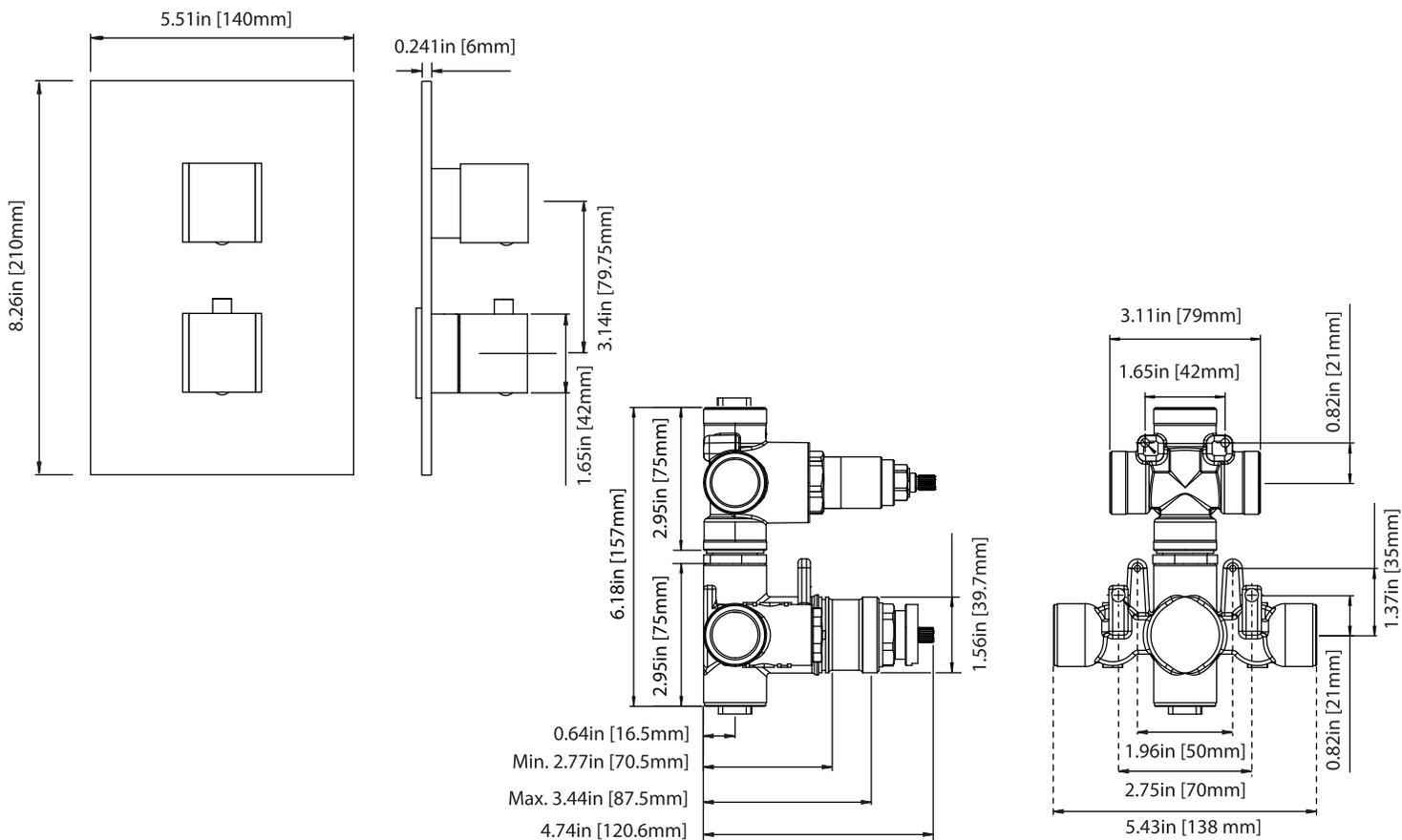
TVH.4420F | 3/4" Thermostatic Valve With 2-Way Diverter & Integrated Volume Control
