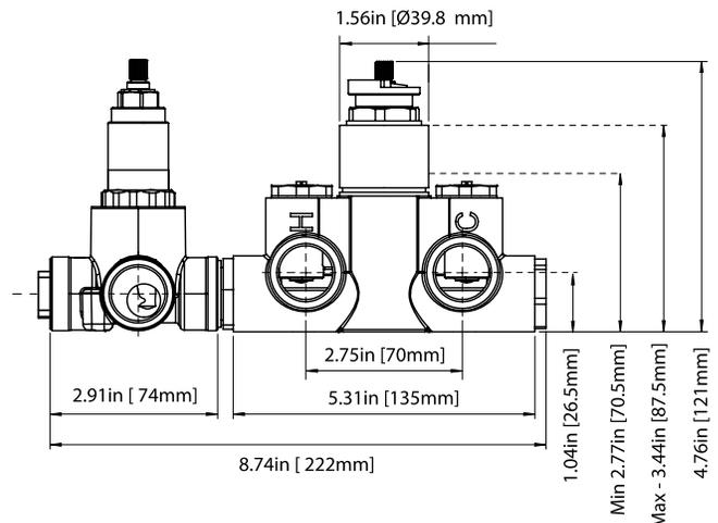
**TVH.2717F | 3/4" Thermostatic Valve With 2-Way Diverter & Integrated Volume Control** Page 2 of 2
