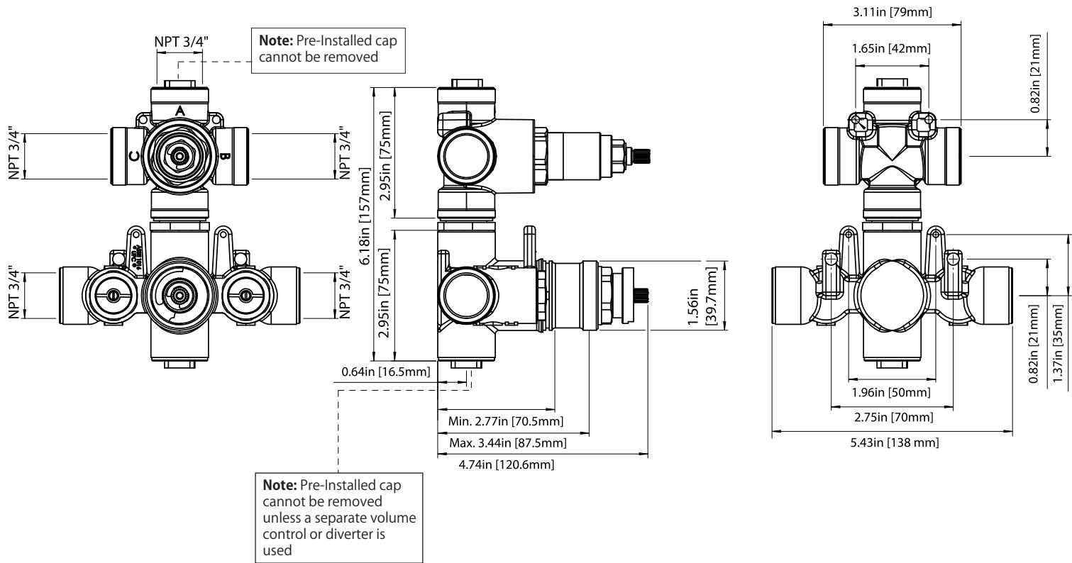
**TVH.4420F | 3/4" Thermostatic Valve With 2-Way Diverter & Integrated Volume Control** Page 2 of 2
