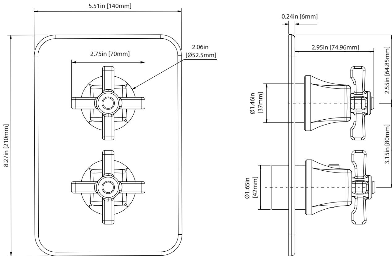
**TVH.4420F | 3/4" Thermostatic Valve With 2-Way Diverter & Integrated Volume Control** Page 2 of 2
