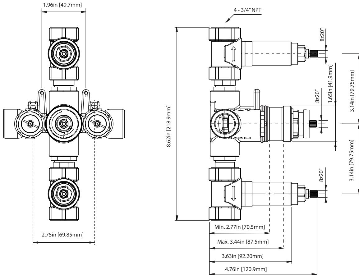
TVH.4401 | 3/4" Thermostatic Valve With 2 Independent Volume Controls Page 2 of 2
